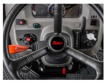
The easy-to-read LED dashboard displays operating data, such as engine speed, temperature, fuel level, time, PTO, etc.
