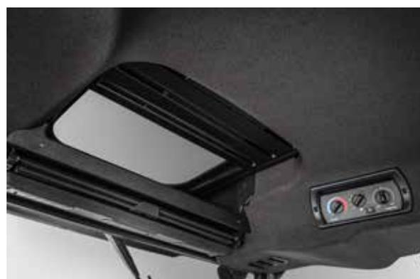
The roof window ensures the good visibility during the work with a front loader.
