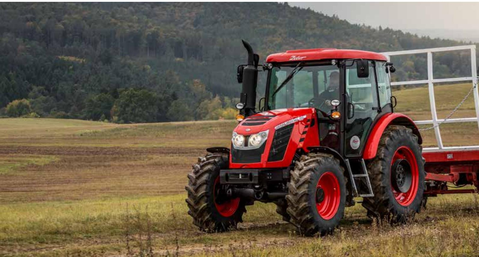
Proxima tractors are universal farm tractors specifically designed for working with agricultural implements, industrial aggregates and for agricultural transport.
