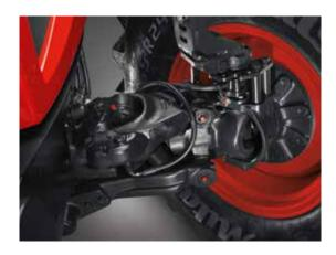
**SUSPENDED FRONT AXLE** The front driven axle of the Forterra HSX and HD models can be optionally suspended. In combination with the suspended cab, this offers a smooth and comfortable drive.
